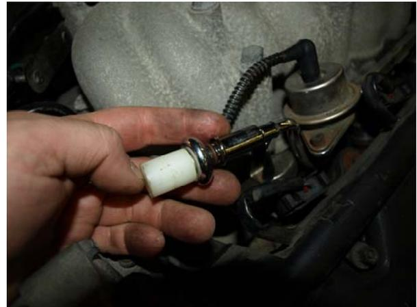
18. Relieve fuel pressure, remove line plug, reinstall return line, and return car to original condition. Put all equipment away.
