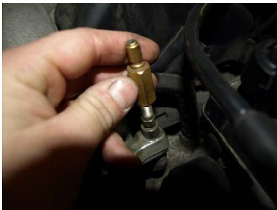
3. Locate the fuel pressure regulator, inlet line, return line, and the Schrader valve. Find the correct adapter to install the gauge on the Schrader valve and install. (Hand tight ONLY!!)
