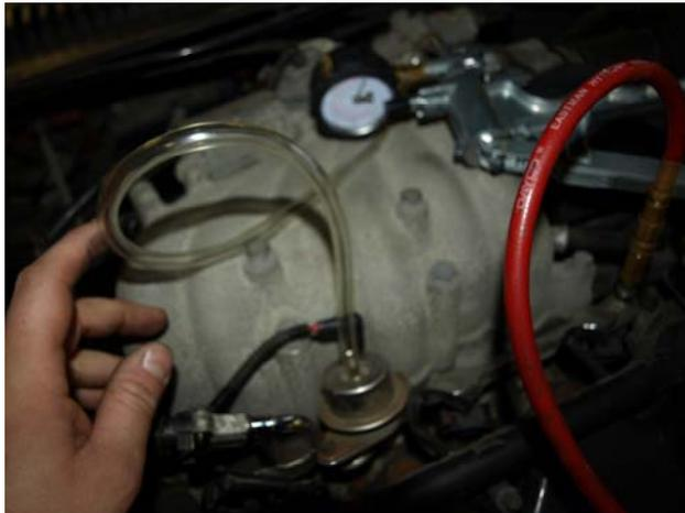
10. Install the hand vacuum pump to the fuel pressure regulator and pump up to 25”hg. Record your fuel pressure.
