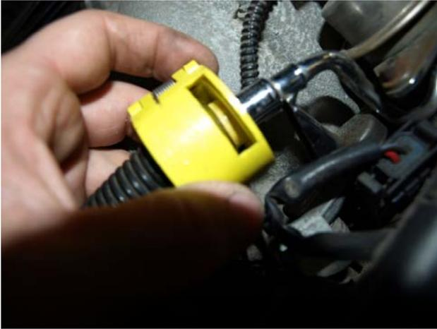
15. Remove the safety clip like in the picture. You will need to find the correct release tool to press on the small garter spring located inside the connector. Mr. Santini will perform a quick demo with the first group.
