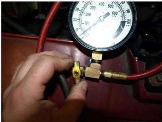
5. Make sure that the pressure relief valve is closed on the gauge set. It should be turned clockwise to close.
